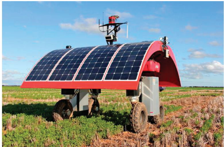
A robot nicknamed the "Ladybird" automatically sprays herbicides and fertilizers. (Photo courtesy of the University of Sydney's Australian Center for Field Robotics)
