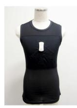
Most of those cloth products are electrically conductive so that electrodes and wires can be placed on them. The biological information of the wearer is collected and sent to smartphones and other apparatuses through a tiny transmitter attached to the chest or elsewhere.
